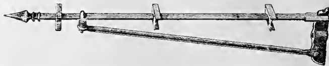
This Cut shows our Punch Fence Line Post with malleable base set on stone coping or blocks. Only one bolt is used for fastening post and brace to the stone.
